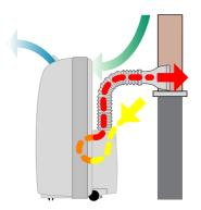
You might decide to install Dolceclima S9 as a fixed unit. Just drill two holes in the wall and use the special installation kit included as a standard. 11.
