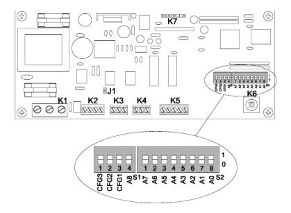
The configuration of these selectors is seen on the ignition of the board; therefore it is necessary to switch off and to switch on when you modify the disposition.
