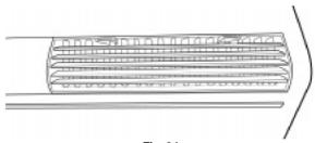
Fig. 34 Control of air flow direction
