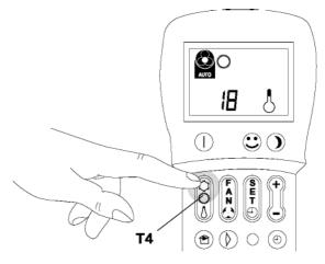
Fig. 33 Heating function (only models with heat pump)
