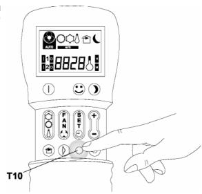
Fig. 41 Resetting all functions of remote control
