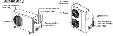
Heat pump model: Cassette Type Air Conditioner for cooling and heating Cooling model: Cassette Type Air Conditioner for cooling
