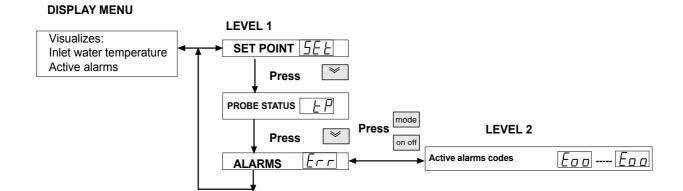
The unit self-protect through safety devices, when any of these safety devices detect an anomaly, shown in the display in order to advice the installer.
