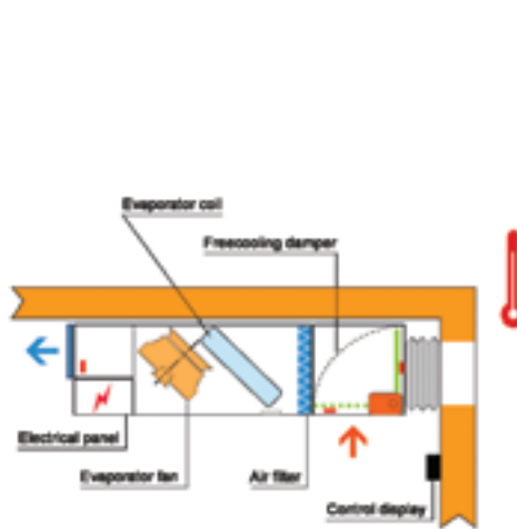
Example of horizontal installation direct expansion mode
