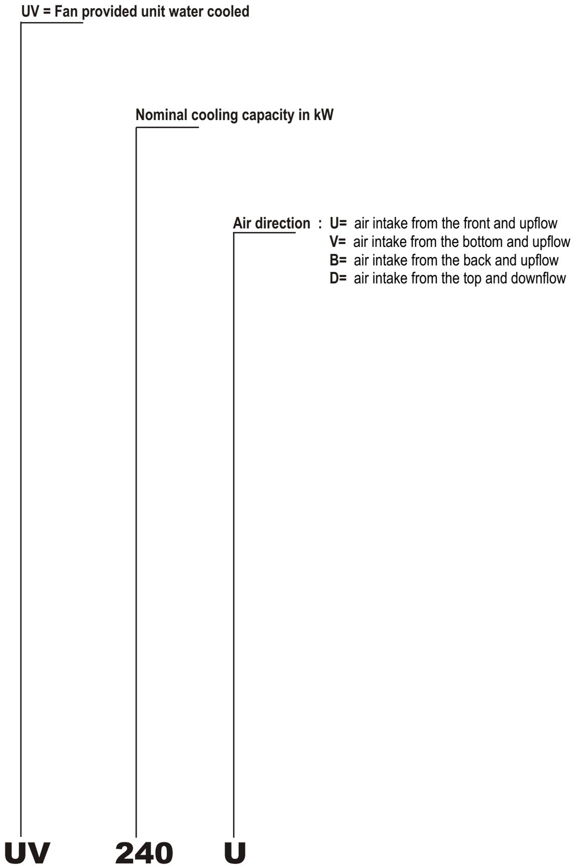
The conditioning units are classified, as shown in the scheme of the previous page, according to the transfer path of the air inside the unit before being discharged into the working space at the desired temperature. Following pictures show the four different configuration, of the air flow system.
