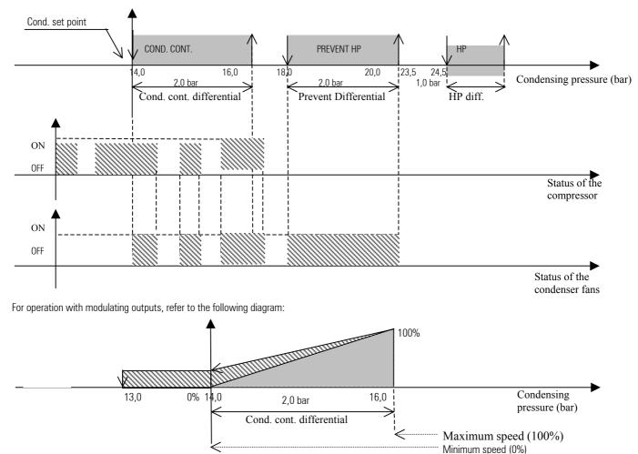
The voltage values corresponding to the minimum and maximum speeds of the fan can be set, between 0 and 10 V; if the minimum value set is greater than 0 V, when stopping the fan is operated at the minimum speed for 1.0 bar below the condensing pressure set point, before switching off, as per the diagram above.
