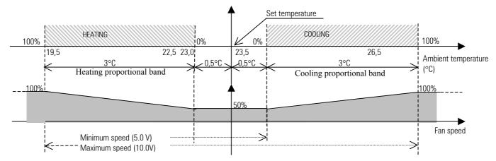
It should be noted how in dehumidification mode the speed is automatically reduced to the default value of 5.0 V (50%), modifiable. The minimum and maximum speed can be set, as default these are 5.0 V and 10.0 V.
