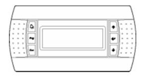
The use of the PGDO\* terminal is very similar to that of the Built-In terminal (access to the loop of screens, on/OFF, etc.). The main menu (PRG button) features the "CHANGE UNIT" item, used to switch between the unit currently connected and the other pCO boards in the pLAN.
