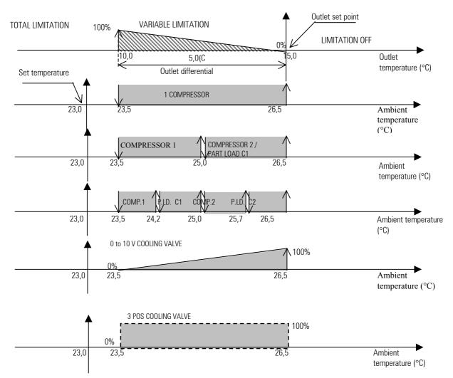
As can be seen, if the outlet temperature is between the outlet set point and the outlet differential, the cooling devices are only partially limited, to a greater extent the lower the temperature.
