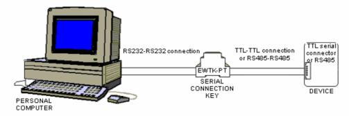
Connections between the PC and the key, and between the key and the CLIMATIC™ 30 shall be carried out without voltage on every CLIMATIC™ 30, and in compliance with safety regulations in force. Electrostatic shocks shall be avoided, particularly on visible metal parts of CLIMATIC™ 30. Check the electrostatic currents are free to flow to ground by means of suitable solutions.
