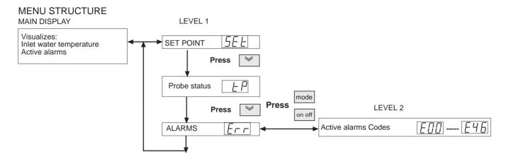
The unit self-protects through safety devices; when any of these safety devices detect an anomaly, this is shown in the display in order to advise the installer.
