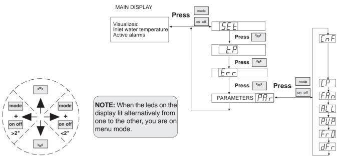
PR Menu of configuration parameters of the unit.
