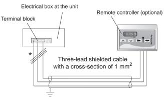
\*Connection to be made by customer MAXIMUM LENGTH 50m
