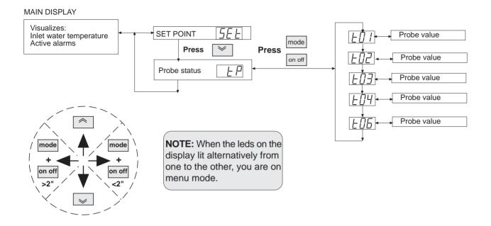
Probe St1 [ [ ] Inlet water temperature.
