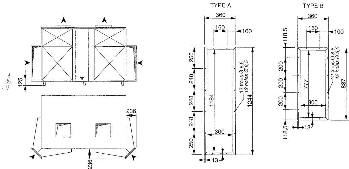
RCCORDEMENT ASPIRATION VERTICALE - VERTICAL INLET CONNECTION
