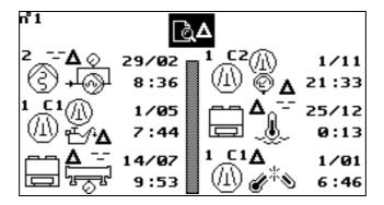
The event log allows recording of the last 24 changes of state related to faults.
