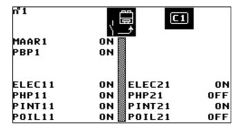
This screen shows the state of all the logic inputs associated with the circuit and its compressors.
