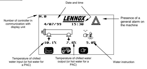
On a machine not fitted with the option "regulation with gradient", the active water instruction (CONSEA or CONSEB) is a variable which can be modified in "modification" mode. In the case of regulation with gradient, the active instruction CONSEA can be modified. However CONSALC cannot be modified, since it is the result of a calculation (see pages 15 and 16).
