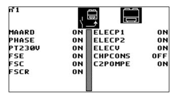
This screen shows the states of contacts which have an effect on the overall operation of the machine (e.g.: remote on / off, circuit breakers for pumps, choice of setting instruction, etc.)
