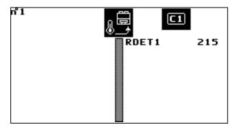
This screen shows the analogue inputs for the refrigerant circuit which are not shown in the refrigerant diagram screens described in § 3.5. (e.g. opening of electronic expansion valve).
