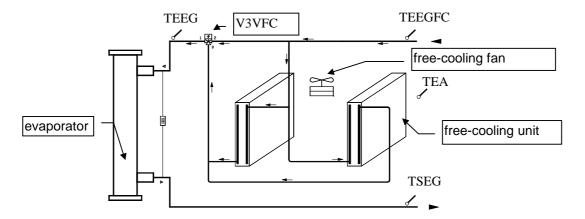
TEEGFC ⇔ Temperature of chilled water input to free-cooling (°C)
