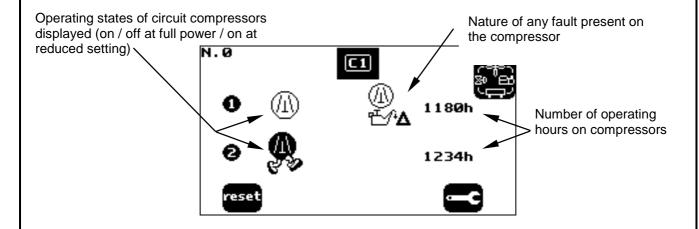
Cause of compressor halt other than a fault (e.g. : anti-short cycle)
