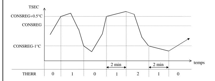
As soon as TSEC becomes greater than CONSREG+0.5°C, capacity is reduced. As long TSEC remains above CONSREG + 0.5°C, an additional capacity reduction cuts in (if applicable) every 2 minutes.
