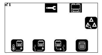
This screen gives access to the values of analogue inputs, logic inputs, TOR outputs, fault counters, and other variables relating to the entire machine (not related to a specific refrigeration circuit). Each variable is identified by its mnemonic.
