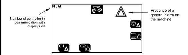
This screen gives access to the operating states of the refrigeration circuits, pumps and machine.
