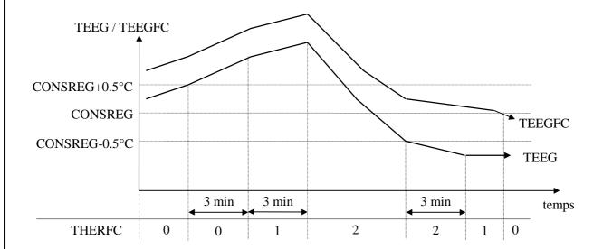
The thermostat is incremented by one stage if TEEG remains greater than CONSREG+0.5°C for over 3 minutes. As long as this condition on TEEG is satisfied, THERFC continues to be incremented by one stage every 3 minutes.
