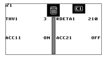
This screen displays the calculated values of significant circuit variables such as the anti-short cycle of compressors, the ventilation thermostat or the order of position given to the expansion valve.
