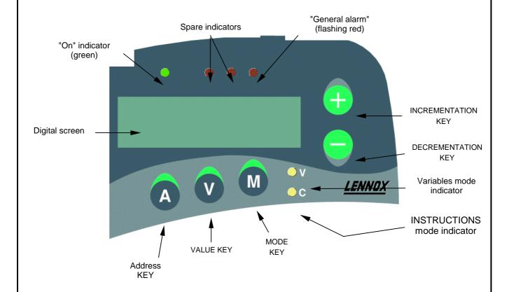
This console is principally used to read and/or modify the values of variables or instructions for the CPU card to which it is connected.
