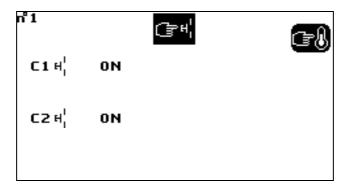
This screen can be used to configure authorisation to switch on each refrigeration circuit, or to keep it switched off, using "modification" mode.
