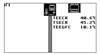
This screen contains the temperatures associated with specific options (e.g. temperatures of chilled water at input to free-cooling or hot water at I/O to a heat recovery exchanger).
