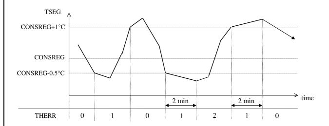
As soon as TSEG becomes lower than CONSREG - 0.5°C, capacity is reduced As long as the TSEG stays lower than CONSREG - 0.5°C, an additional capacity reduction cuts in (if applicable) every 2 minutes.
