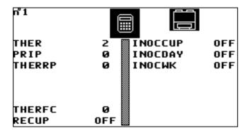
This screen gives the values of calculated variables which apply to the entire machine. (e.g.: priority status for pump operation, pump operation, idle functions, etc.)
