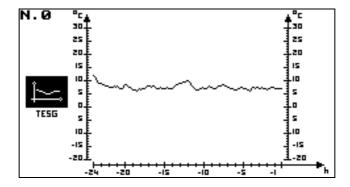
The monitoring frequency for the temperature of chilled water output (or hot water for a PAC) is 10 minutes, over a complete 24 hour cycle. The console therefore memorises the last 144 values of the monitored variable.
