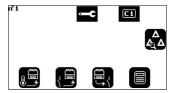
This screen gives access to the values of logic inputs, fault counters, TOR output and other variables describing the selected refrigeration circuit. Each variable is identified by its mnemonic.
