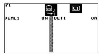
This screen displays the state of the actuators which control circuit components other the compressors, whose operation has already been described in operating states for circuits (see § 3.4.).
