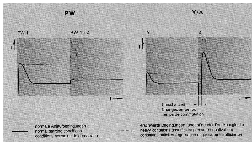
You can see that the use of part winding compared to open transition star delta offers an overall reduction in starting current. In part winding the introduction of the second stage of the motor winding takes place without stopping the motor. On star delta the motor is stopped and as a result there is a significant peak in inrush current in delta at that time. On star delta the initial inrush current is smaller than part winding initial inrush.
