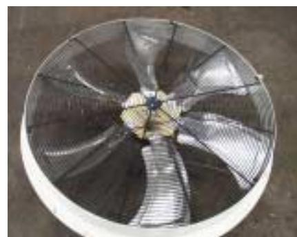
The new Hush tone condenser fan features six aerofoil pitched blades statically and dynamically balanced. The blades have sickle end section in a bell mouth orifice for reduced noise and improved performance. This fan design is unique to **LENNOX**. The fans are direct driven via a three phase motor with permanently lubricated ball bearings. The motors are designed for external operation and are available with different speeds with the option of two-speed motor.
