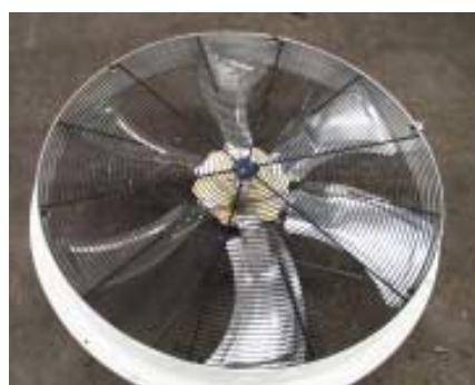
The new Hush tone condenser fan features six aerofoil pitched blades statically and dynamically balanced. The blades have sickle end section in a bell mouth orifice for reduced noise and improved performance. This fan design is unique to **LENNOX**. The fans are direct driven via a three phase motor with permanently lubricated ball bearings. The motors are designed for external operation and are available with different speeds with the option of two-speed motor.
