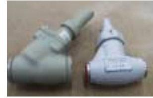
Compressor Isolation valves
