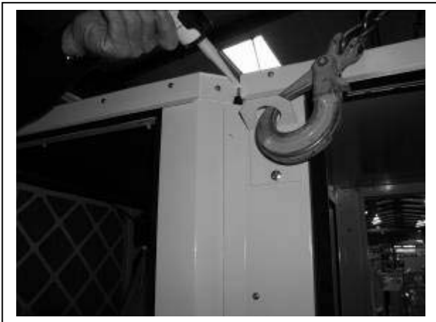
Putty very carefully on the roof side and then on flange sides
