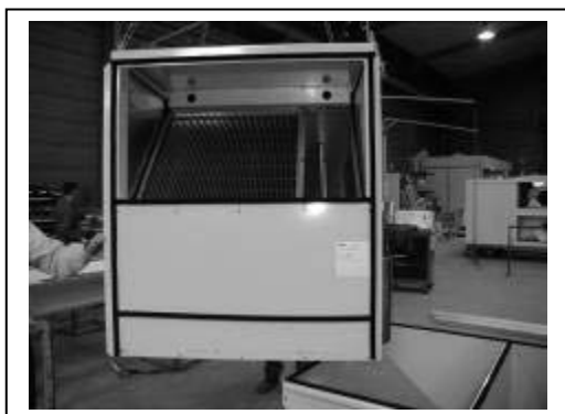
Bring the module on the support. Check the good shape of the 20 x 10 black gaskets.
