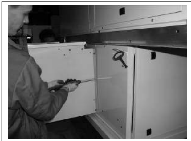
The sheet metal return must inside the frame slot.
