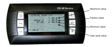
≥: to quickly increment or decrement the setting, hold the "↓" or "↑" keys during some time.
