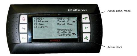
To access to alarms history, press the "ALARM" key when you are in the main menu (**0000**). The CLIMATIC 60 saves up to the last 32 alarms. An active alarm is signaled by the symbol "\*" whereas an alarm inactive is symbolized by the "=".
