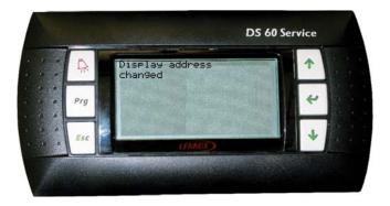
5. Use the "\", "\" keys to select the desired address of CLIMATIC 60. CLIMATIC 60 address must be at the address "1" except if there is several units linked. The next screen is displayed.
