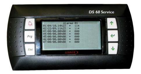
The menus are organised in arborescence tree with submenus as per the scheme hereunder. The actual menu is identified by a 4 digit number between brackets displayed in the top left corner of the screen.
