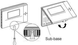
3° To fasten the rear part of the box to the wall, place the hole in the centre of the box over the cables for the control of the instrument which come out of the wall. The placement of the mounting holes has been designed to allow the instrument to be fixed onto a box conforming to standards CEI C.431 - IEC 670. If this is not available, use the mounting holes on the shell as a guide for drilling holes into the wall and then use the screw and plug kit supplied.
