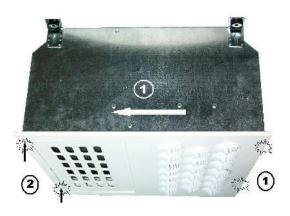
Raise the diffuser towards the unit, the locating lugs should clip to the diffuser, two clicks should be heard (2), the diffuser can now support itself.
