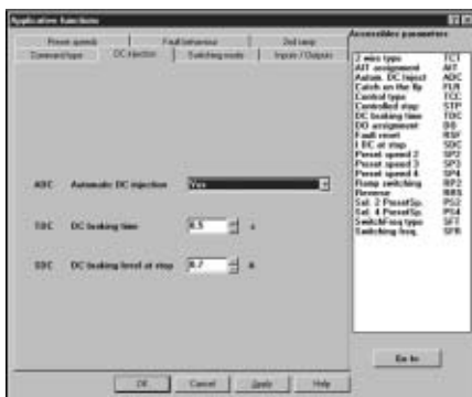
Adjustment of the "d.c. injection" function using the PowerSuite software workshop for PC
