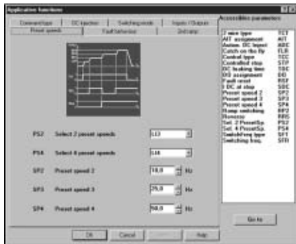
Adjusting the preset speeds with the PowerSuite software workshop for PC
