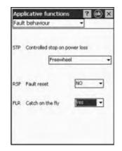
Adjustment of the behaviour at a fault with PowerSuite Pocket PC
