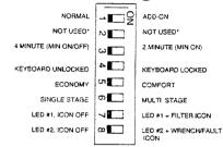
\*NOTE: Switch #2 must be left in the OFF position.
