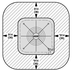
NOTE—1219 mm (48 in.) clearance required on top of unit. \*NOTE—One side must be 914 mm (36 in.) for service. Two of the remaining three sides may be 305 mm (12 in.).
