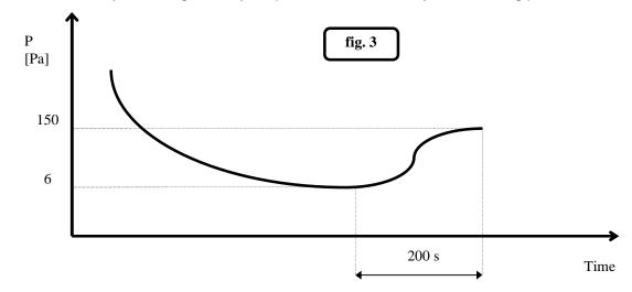
The **fig.3** represents a vacuum cycle and an optimal subsequent pressure rise for the refrigeration devices we manufacture.
