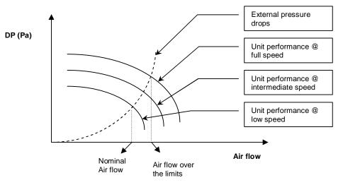
In the EC fans the rotation speeds are selected with different values of the control tension (0 - 10V). The right value of the control tension has to be set by keyboard, considering the AESP requested on site. If the unit is equipped with the "air flow control" option, the mp manage the fan speed in order to obtain the required air flow (Air flow set-point).
