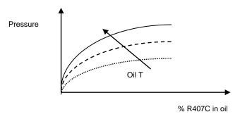
The diagram above illustrates a specific property of gases [Charles' Law], which are more soluble in liquids as the pressure increases but less soluble as the temperature increases: if the oil in the sump is held at a constant pressure, an increase in temperature will significantly reduce the amount of refrigerant dissolved in it, thus ensuring that the desired lubricating function is maintained.
