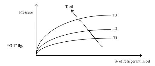
If the oil in the sump is held at a constant pressure, an increase in temperature will significantly reduce the amount of refrigerant dissolved in it, thus ensuring that the lubricating function desired is maintained. The problem of inadequate lubrication occurs if the crankcase is not duly heated, above all after seasonal
