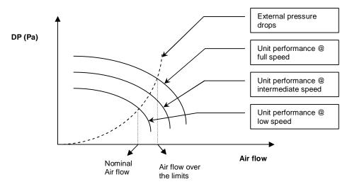
The fan speed has to be selected according to the enclosed table by using the manual switch installed in the E-Panel and/or by changing the wire connections of the autotransformer for different selection than the four already available on the manual switch.
