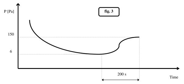
The figure **fig.3** represents a vacuum cycle and an optimal subsequent pressure rise for the refrigeration devices we manufacture.
