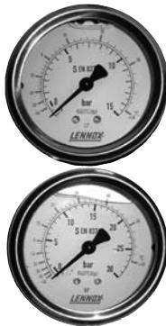
Liquid filled gauges that measure the evaporating Low pressure (LP) and condensing high pressure (HP) on each refrigerant circuit. Gauges are «glycerin» filled to damp gas pulsation and are mounted externally. The gauges are compound gauges that display the saturated refrigerant temperature for the refrigerant R407C.
