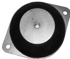
Elastic supports (Rubber) made of 2 flat and parallel frames, connected together via a rubber ring, fixed under the unit at the points specified by our technical drawings. Reduces the transmission of vibration to the ground and the general sound level. The diameter and strength vary in accordance with the model. Delivered loose not fitted. This type of mounts is not adapted to concrete slabs. Supplied loose.
