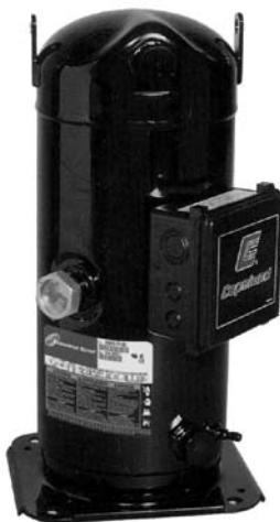
Scroll compressors are comprised of two identical scrolls mated together to form concentric spiral shapes. Note the absence of seals between the two scrolls. The Scroll design maintains consistent volumetric output even without seals. Absence of dead space, resulting in a volumetric efficiency approaching 100% for the compressor. Fewer moving parts, leading to lower failure rate.
