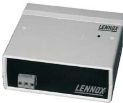
This is an additional microprocessor board that is able to provide information using JBUS protocol to allow exchanges between the climatic control system and an external BMS system. Lennox has existing protocols in place with most BMS companies but this option can require additional support above the basic costs of the interface module. Supplied loose.
