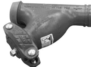
Water strainer/filter is to be installed upstream on the water inlet to protect the evaporator and condenser from any possible impurities (1 mm efficiency). It is recommended for shell and tube heat exchangers and must be fitted on units with plate heat exchangers. Supplied loose.
