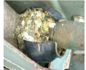
Galvanic corrosion under the plastic sleeve.
