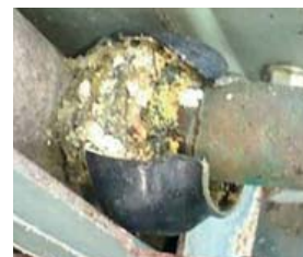
Galvanic corrosion under the plastic sleeve.
