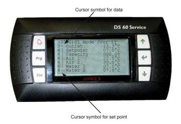
To modify a setting, move the cursor on the desired item and press the " $\leftarrow$ " key. A new screen displays information concerning this set point. To modify it, use the " $\downarrow$ " and " $\uparrow$ " keys and validate by pressing the " $\leftarrow$ " key. If the setting is customizable according to the schedule mode, press the "PRG" key to select different value for the Day, Day I, Day II & Night modes.
