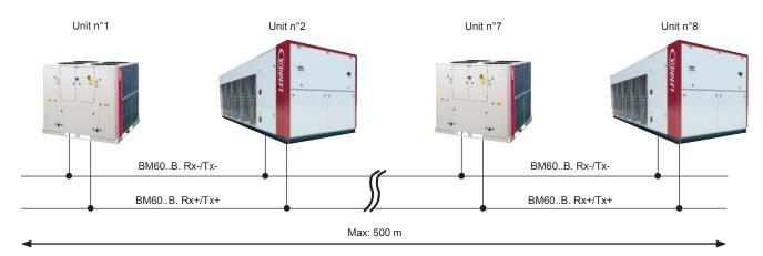
The pLAN bus is connected to CLIMATIC™ 60 on the J8 connector of board BM60. A star connection is not recommended. For an optimum operation it is advised to connect a maximum of two cables per unit.
