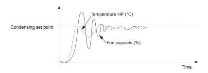
In order to optimise the performance of the unit, the condensing temperature is set according to outside air temperature and tries to maintain a delta of 12°C (only for unit with electrionic expansion valve).
