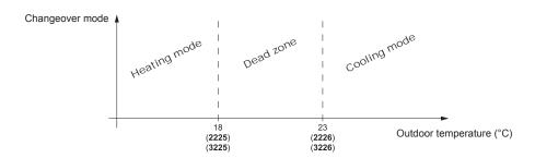
If the outside temperature is below the setting value (2225) or (3225), the unit will operate as a heat pump. If the outside temperature is over the setting value (2226) or (3226), the unit will operate as a chiller.
