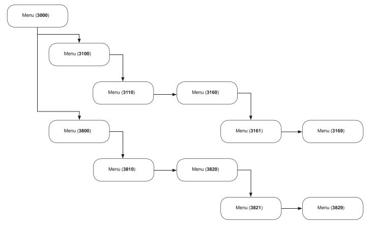
The " $\downarrow$ " and " $\uparrow$ " keys are used to move the cursor on the desired item. Then use the " $\leftarrow$ " key to enter in the selected submenu. To escape a menu use "ESC" the key.
