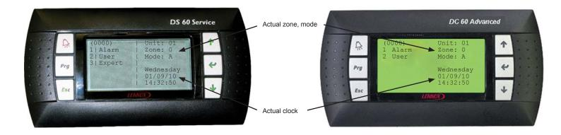
To access to alarms history, press the "ALARM" key when you are in the main menu (**0000**). The CLIMATIC™ 60 saves up to the last 32 alarms. An active alarm is signaled by the symbol "Alarm" whereas an alarm inactive is symbolized by the "." To reset the current active alarm(s) press the "ALARM" key.
