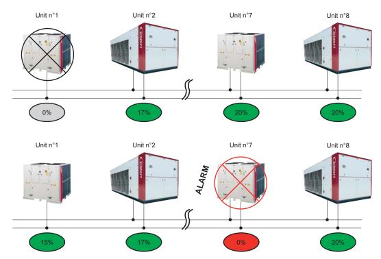
The CLIMATIC™ 60 manages also the rotation between the declared units . In "Cascade" mode, that means that the first unit to start will change every week. In "Rol.Backup" mode, the unit in "Backup" is swapped every week.
