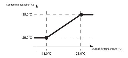
Note: this functionality can be disabled if the selected setting (3545) is different from the factory value. In this case the condensing set point is the new selected value.
