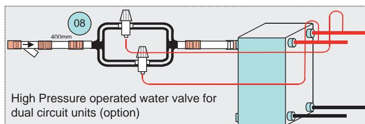
High Pressure operated water valve for dual circuit units (option)
