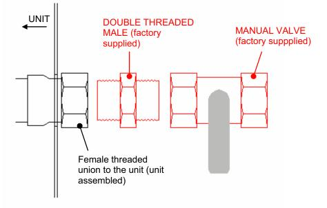
Then, weld a threaded male union (or a double threaded male and a female threaded union just like the connection done in the unit) and connect the water suction/discharge pipe to the valve. The valve keeps the pipe connection just like it was in the unit.
