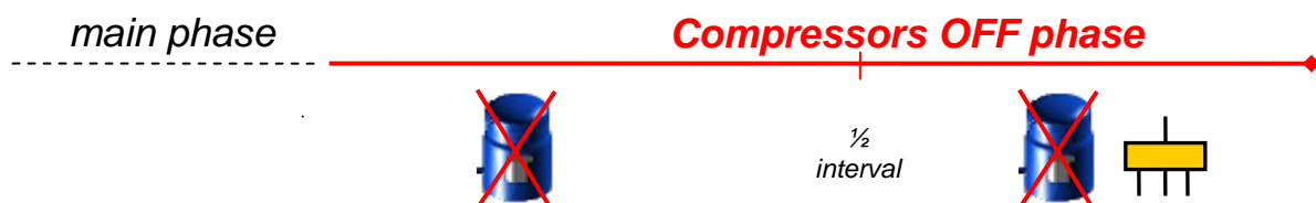
Figure 22: Devices controlled by override in the case of “Compressors OFF when Defrosting Ends”
